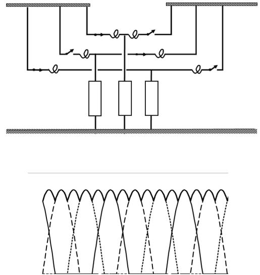
Figure 2 Parallel MMDCT's to smooth input and output waveforms
