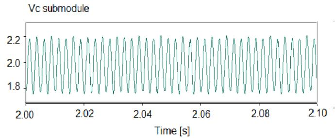
Figure 7 Steady state Input and output currents and capacitor column voltage of each branch at 1 pu power transfer.
