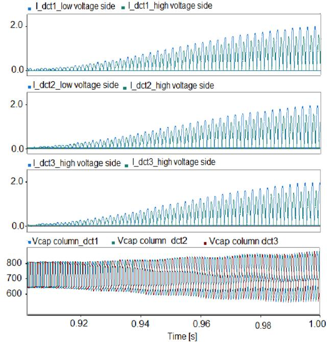
Figure 6 Input and output currents and capacitor column voltage of each branch during power changing from 0 to 1 pu
