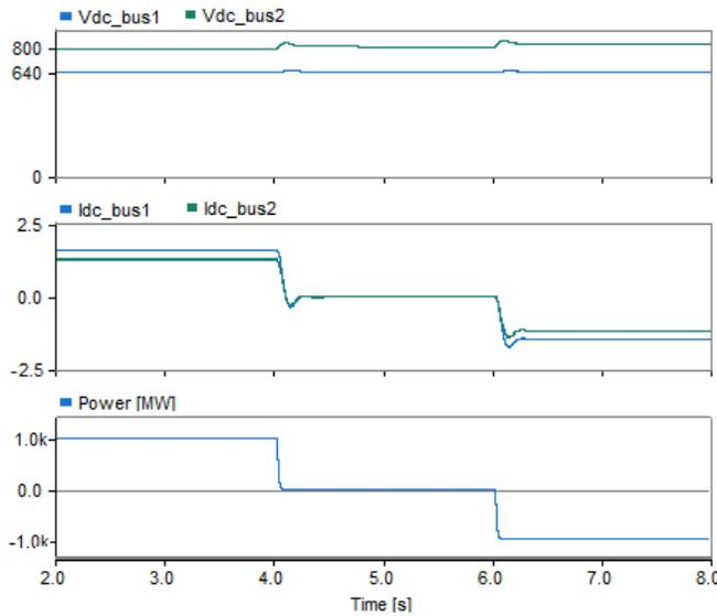
Figure 5 – Dc voltage, current, and transmitted dc power at bus 1 and
