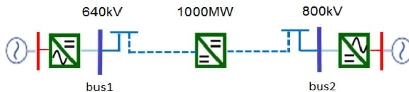
Figure 4 – Interconnection of two large HVDC lines via MMDCT
