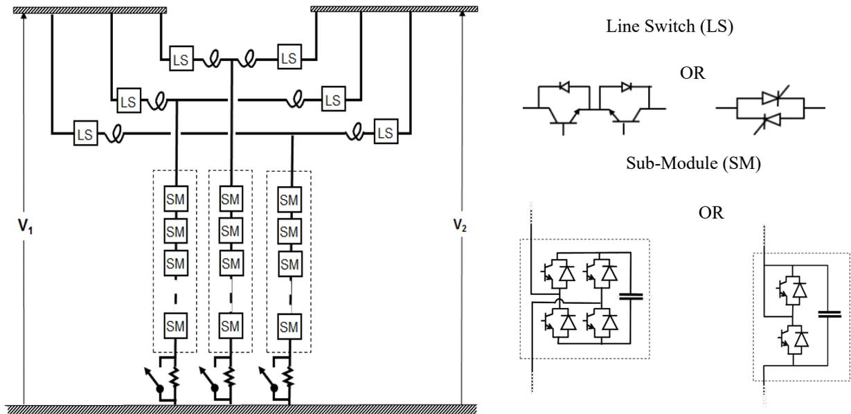
Figure 3 – Circuit diagram of the MMDCT. Options for line switches (LS) and sub-modules (SM) in capacitor column are shown
