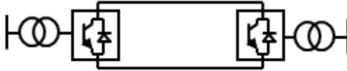
Figure 1 Unearthed, or high resistance earthed, Symmetrical monopole
