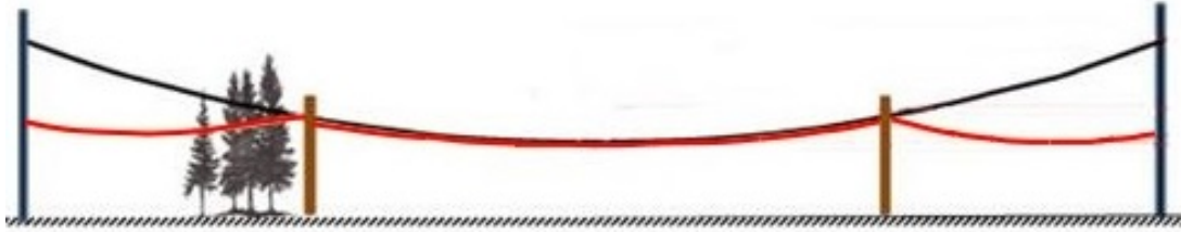
Figure 7: How a low profile reduced span transmission line may appear comparing a 400 m span to a 200 m span. [2]
