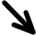
Figure 7.19 Symbol for the E-TRAN arrow, which indicates that a bus continues on another page.
